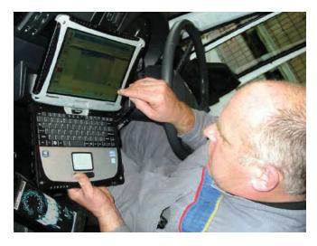
foreman Cliff Green. "But Easy told me immediately that it was a blown fuse. Not everyone would think of checking a fuse before testing the sensors, so the system potentially saved a considerable amount of time and cost."
